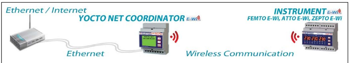
The Yocto net Coordinator E-Wi is connected wirelessly to an E-Wi device as the Femto E-Wi, l'Atto E-Wi, lo Zepto E-Wi, etc.
