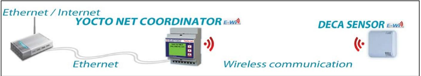
The Yocto net Coordinator E-Wi connected wirelessly to a Deca Sensor E-Wi which measures temperature, humidity, luminosity, etc. The Deca Sensor E-Wi can be powered by a battery or through an external power supplier.
