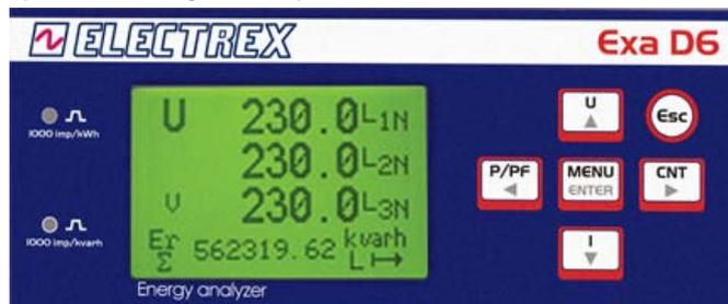
The 6-key Joystick keypad and the menu column on the display for configuring provide a simple and rational instrument use. In addition the initial page displayed when the instrument is turned on can be defined by the user.
