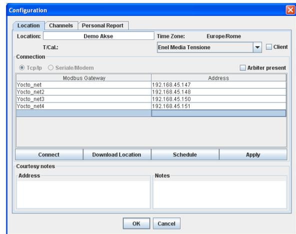
To each location can be associated a different way of communication with their specific personalization. The data download may be manual or automatic through the definition of the agenda. You can activate a password to enter the configuration menu in order to protect it for external unauthorized use.
