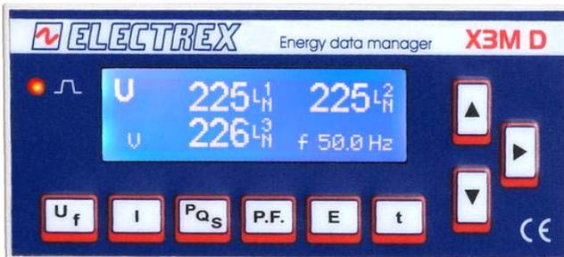
9 keys, with clear indication of their function, make the instrument's use simple and intuitive. A Led indicator, pulsing with a frequency proportional to the active import power, is also provided on the front panel for field calibration verification by means of external optical devices.
